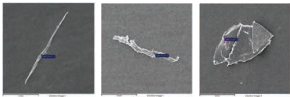
SEM images of different types of microplastics obtained
